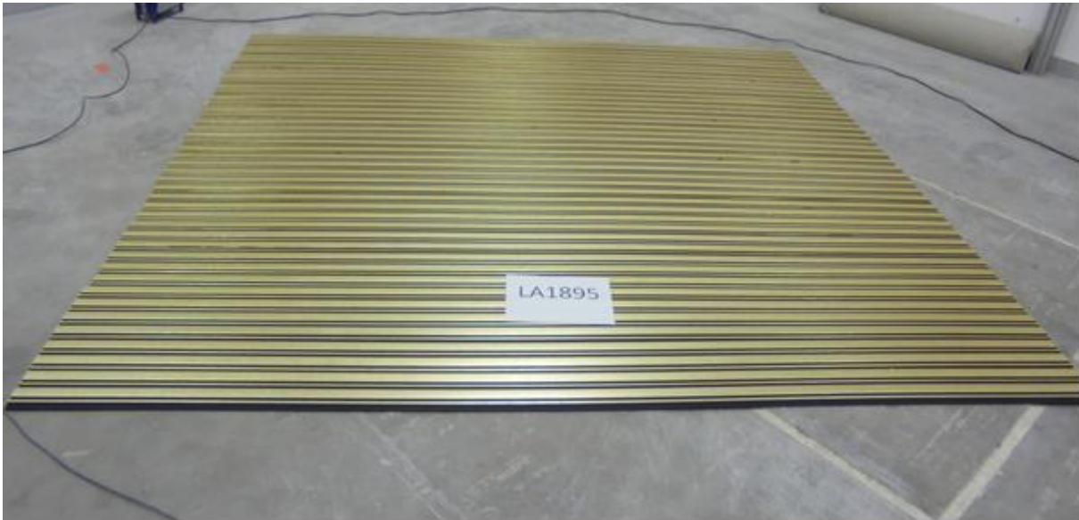
Fig. 1. A photo of tested object No. LA1895 in Laboratory's reverberation chamber
